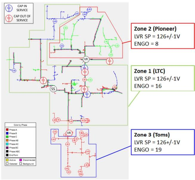
Figure 8: Switx City Voltage Regulating Zone
