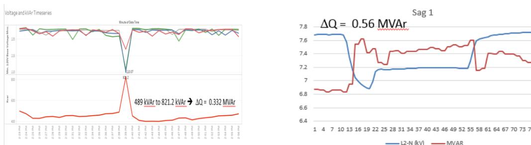
Figure 8: Sag event collected by DVC (voltage left), response rate captured by voltage and kVAr plot on the right as recorded by PQube at the substation
