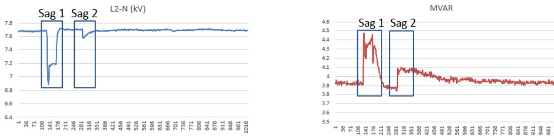
Figure 7: Sag event collected on substation (voltage left), (kVAr right)
