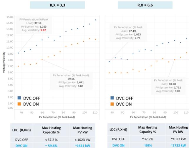
Figure 8. PV Hosting Simulation results for Waimanalo Beach
